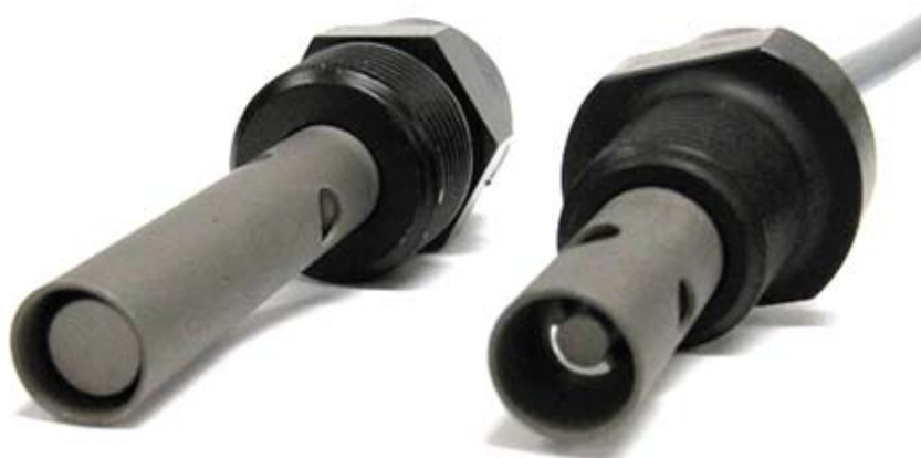
Figure 5. 0.01 cm -1 constant (left) and 0.1 cm -1 constant (right) resistivity sensors comparing electrode length and spacing.
